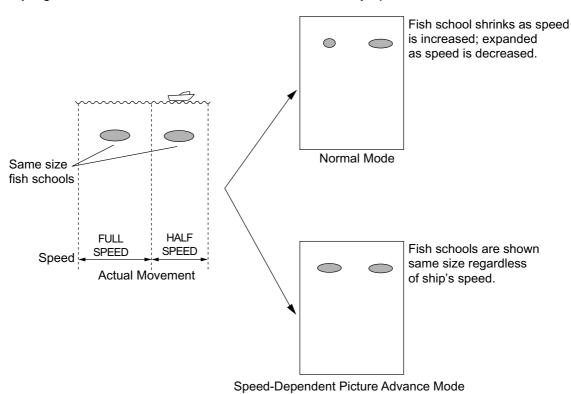
How the speed-dependent picture advance mode works
